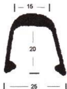
TR SECTION 3291 - only available in 8 metre lengths Standard Slotting 32mm x 13mm at 105mm centres- AP291 Fairlead Joiner 064 & Track End 068 castings available
